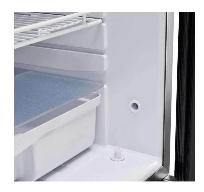
The easy-fix system allows a simpler and faster built in installation than the traditional system. The installation takes place by inserting fixing screws directly from inside the product to the walls of the cabinet through guide holes that prevent the refrigerator side insulation from breaking. The easy-fix system also eliminates the need to apply mounting brackets.
